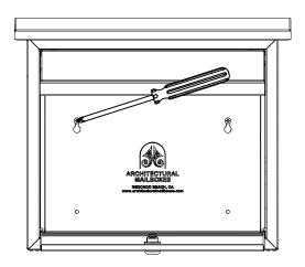
While the mailbox is hanging on the top screws, insert the remaining two screws into the bottom holes and secure with a screwdriver.
